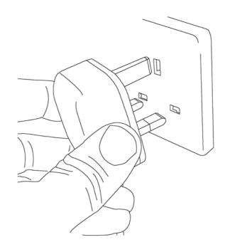
**4.** Finally, plug the mains cable <u>directly</u> into a wall outlet and switch on the socket if applicable (UK mains plug shown).
